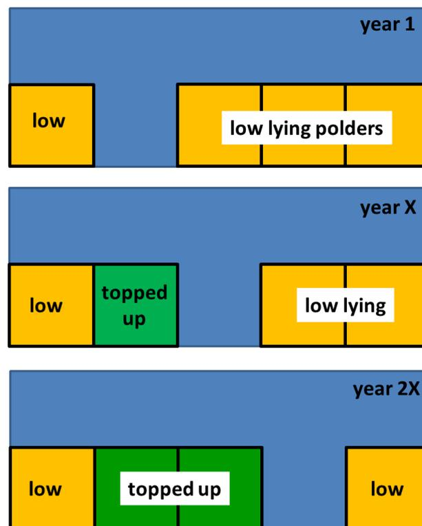
Figure 8.3 Schematic of the Temporary Open Polder concept (TOP polder).
