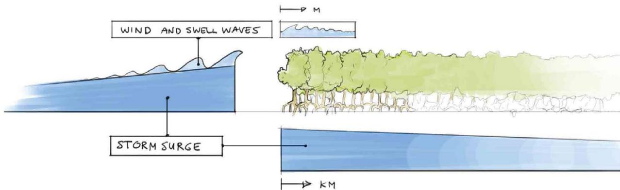
Figure 6. The propagation of the wind and swell waves along the coastline, both in the presence of vegetation and without (Spalding et al., 2014).
