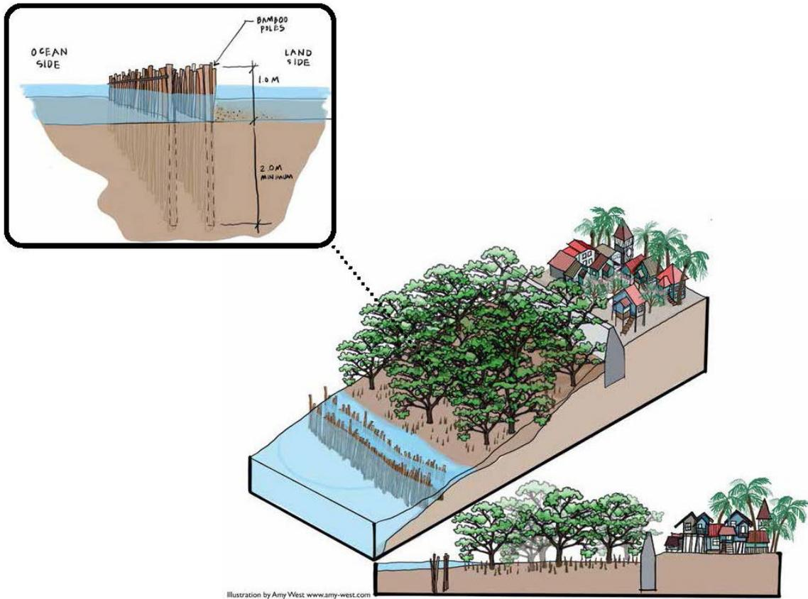
Figure 8. Permeable bamboo fences to dissipate wave energy
