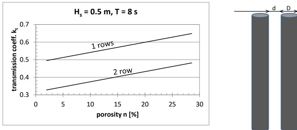
Figure 15.1 Indicative transmission coefficient  $k_t$  as function of fence porosity  $n$  for a single and double row fence and as a function of water depth  $h$  and wave height  $H_s$ , and definition of fence parameters (frontal view).
