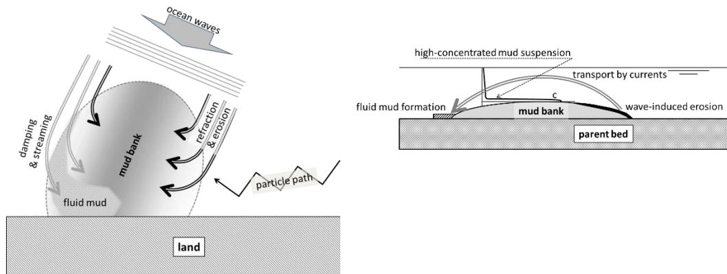
Figure 4.7 Schematic of flows and waves around a mudbank and fine sediment transport (G. current = Guiana current; grav.circ. = gravitational circulation).
