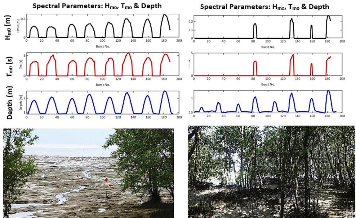
Figure 6.3 Wave Heights, Wave Periods and water depths for (right) 1.6 km offshore and (left) at location approximately 25 - 30% of the fringe width (from the edge) along the Chateau Margot coast, Guyana.
