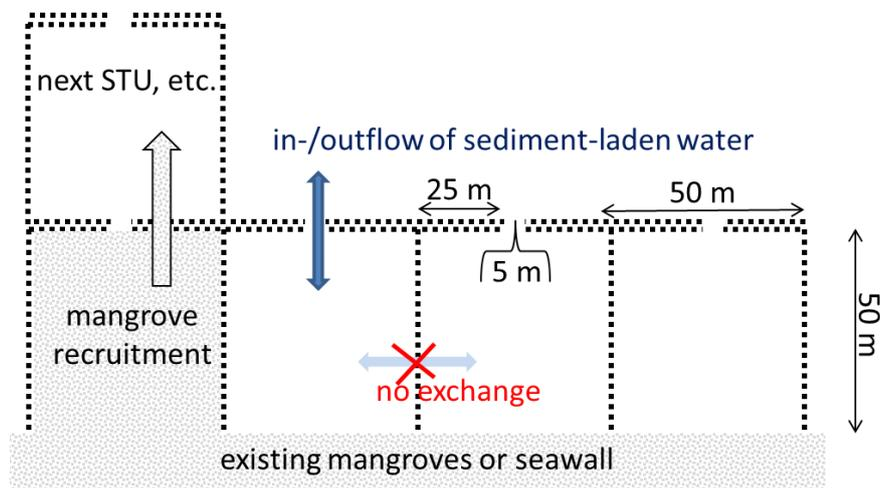
Figure 15.2 Schematic of serial 50×50 m<sup>2</sup> STU deployment.
