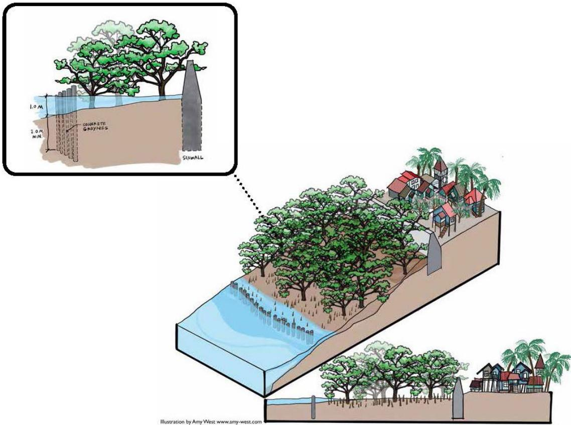
Figure 9. Permeable concrete groynes
