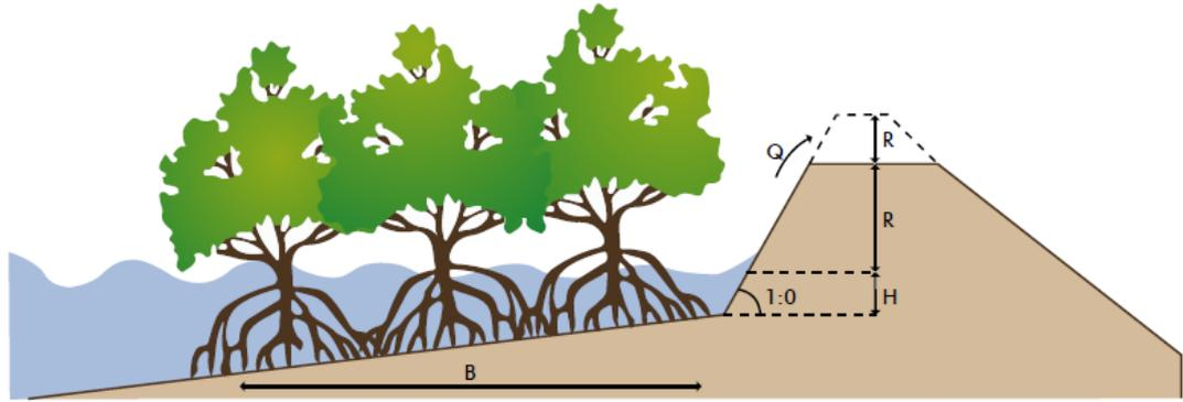
Figure 2.2 Combination of mangroves with a seawall or levee and the parameters influenced by the presence of mangroves (World Bank, 2017)
