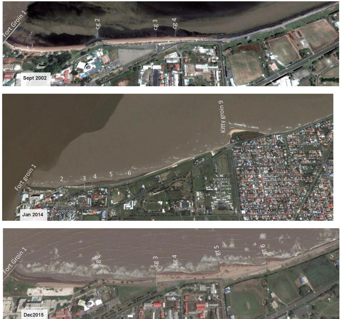
Figure 7.7 Beach development near Georgetown (Google Earth images) at two different spatial scales to visualize coastal response to natural development and cutting of Kitty Groyne mangroves.
