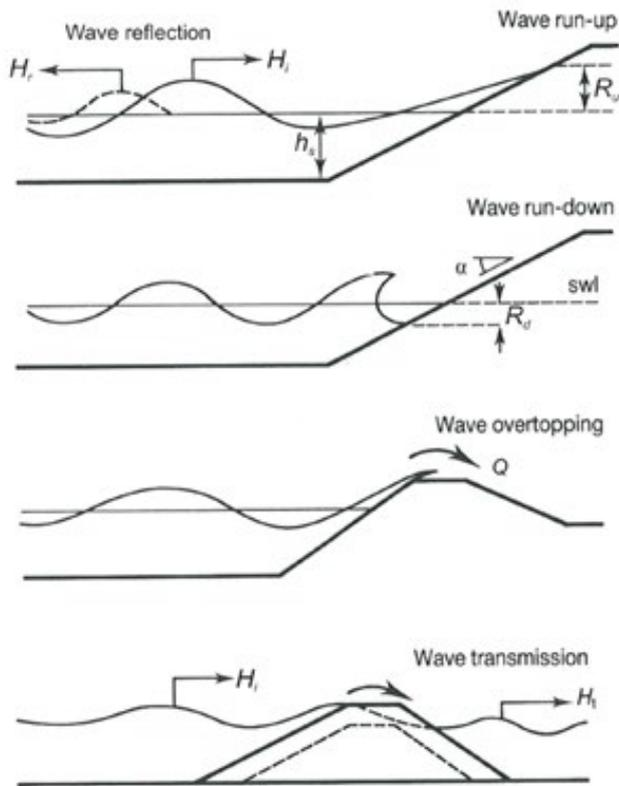
Figure 14. Hydraulic interactions related to waves and parameters definitions (copied from the Rock Manual (CIRIA, 2007))
